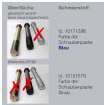
Bolt preparation (Liebherr information sheet TI 723/2018)
